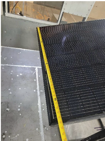
Figure 22: Solar panels width, Run 6 through 8
