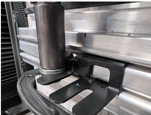
Photo 11: "H" bracket deformation post test
