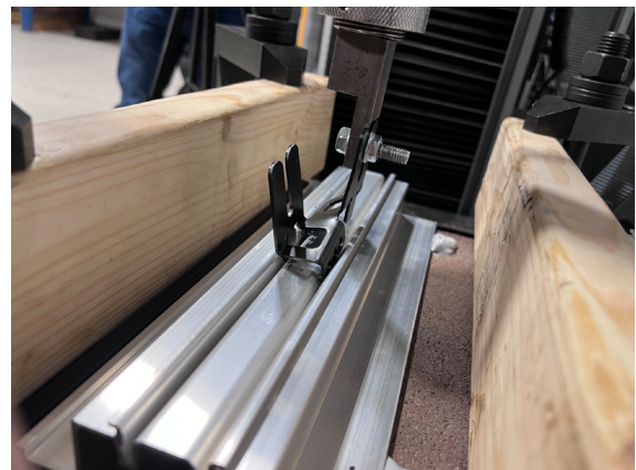
Photo 6: "H" bracket deformed and slipped out of Multiballast DB base test #2
