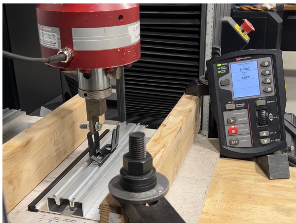
Photo 5: Bolt slipping out of "H" bracket
