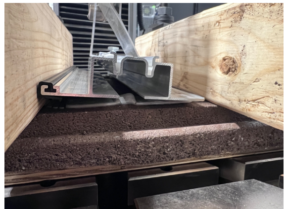
Photo 12: Tension test #4 adhesive failure, aluminum to adhesive
