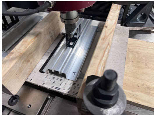
Photo 3: Tension test, setup #1
