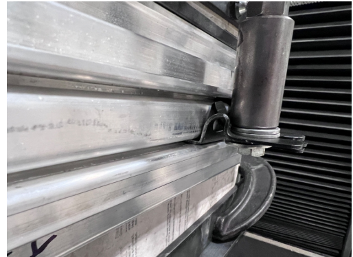
Photo 10: "H" bracket deformation post test
