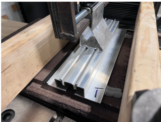
Photo 9: Tension test, setup #3
