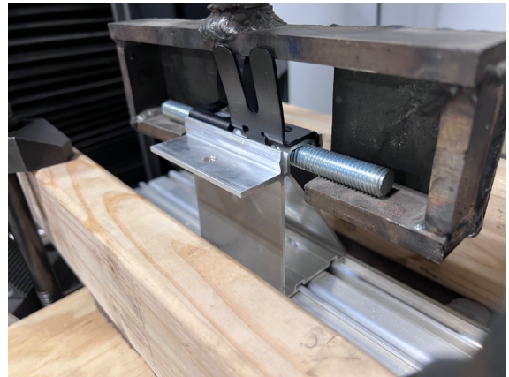
Photo 8: Tension test setup with riser bracket
