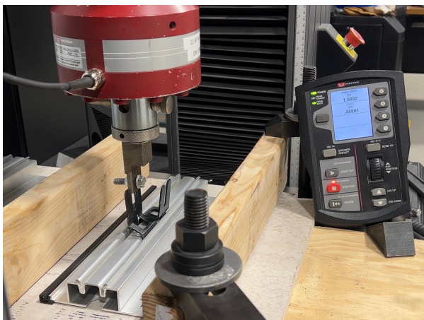
Photo 5: Bolt slipping out of "H" bracket
