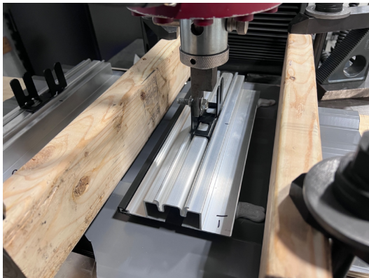
Photo 3: Tension test, setup #1
