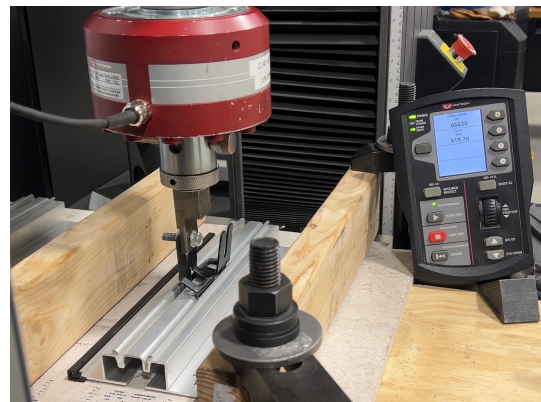
Photo 4: Approximate load before bolt slipped, 520 lbf
