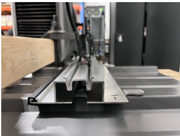
Photo 5: Tension test #1 "H" bracket slipped out
