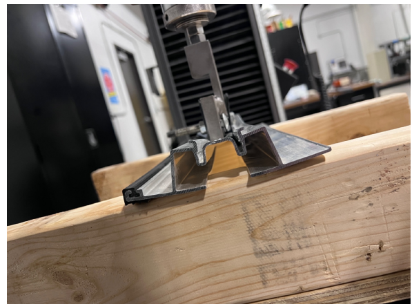
Photo 6: Deformation post testing
