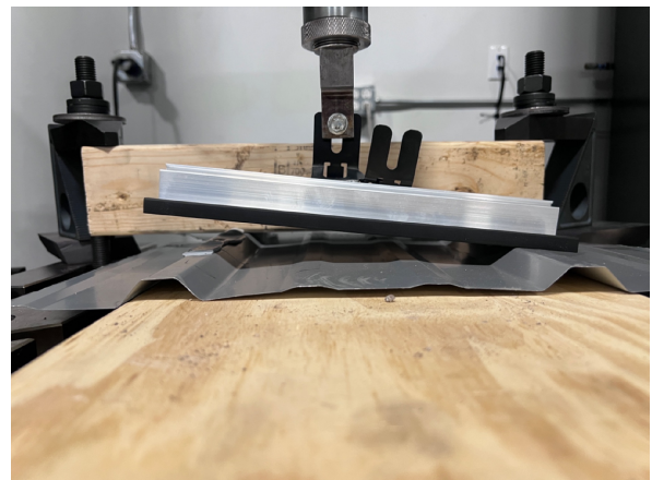
Photo 6: Tension test #2 adhesive failure, aluminum to adhesive interface
