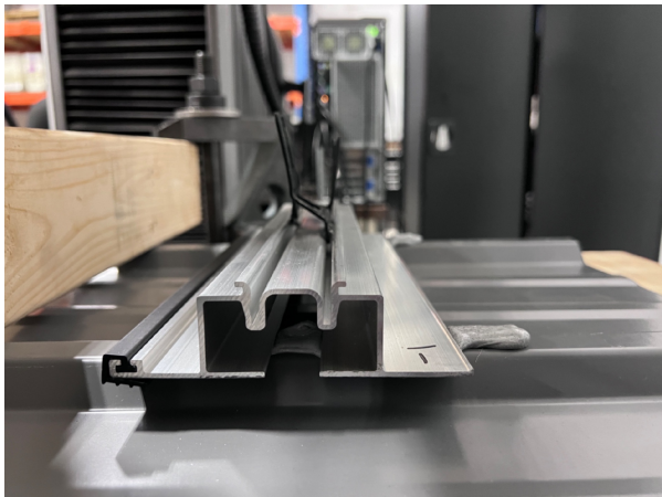
Photo 5: Tension test #1 "H" bracket slipped out
