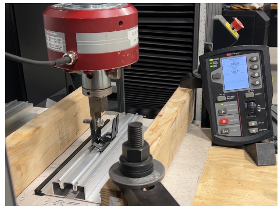
Photo 4: Approximate load before bolt slipped, 520 lbf
