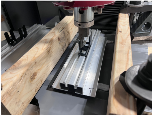
Photo 3: Tension test, setup #1
