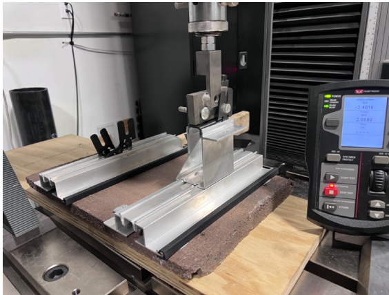
Photo 13: Compression test setup
