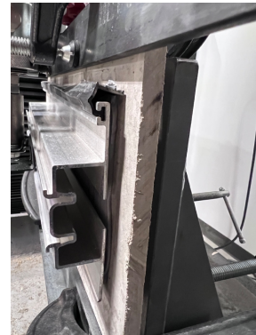
Photo 12: De-bond between the aluminum to adhesive interface
