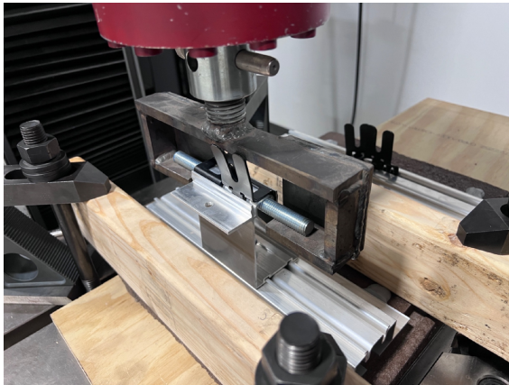
Photo 7: Tension test setup with riser bracket
