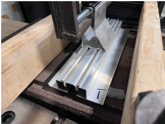
Photo 9: Tension test, setup #3
