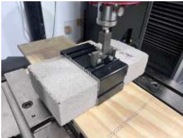
Photo 5: Compression test, setup #2
