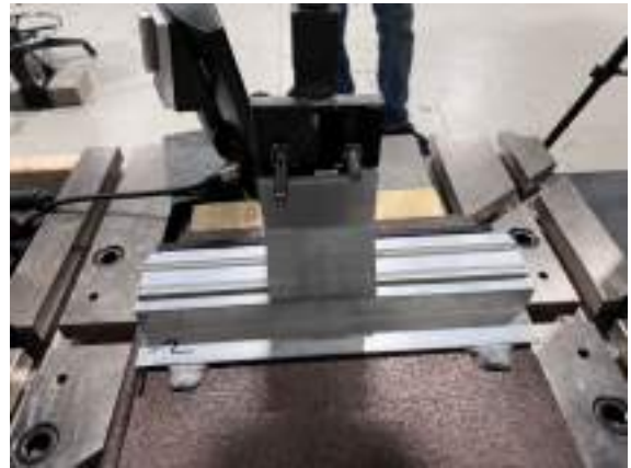
Photo 14: Compression test setup
