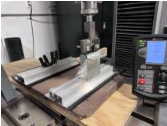
Photo 13: Compression test setup
