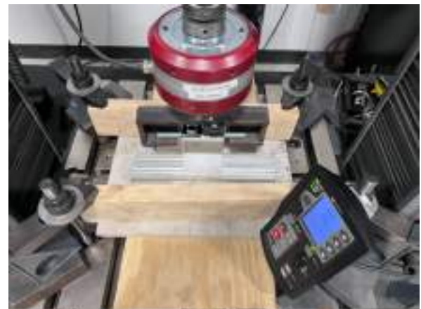
Photo 6: Tension test, setup #2
